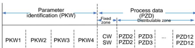
Figure 2-4 PROFIBUS-DP information frame data structure
