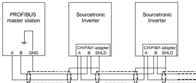
Figure 2-3 PROFIBUS bus connection
