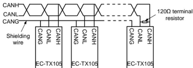
Figure 3-1 Electrical wiring diagram
