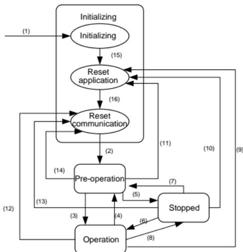
Figure 3-3 NMT state diagram
