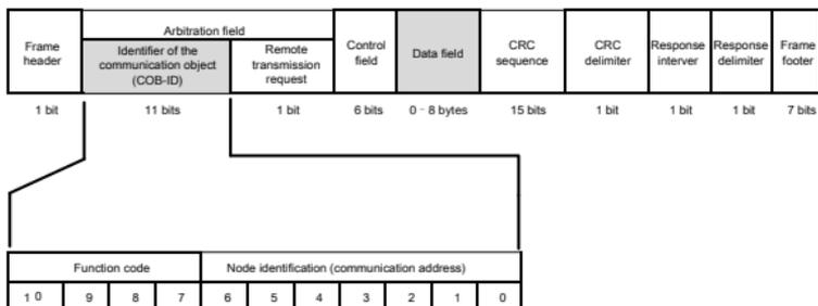
Figure 3-2 Packet structure
