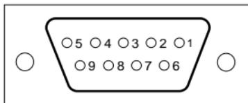
Figure 2-1 Plug of the connector
